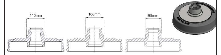
The spigot size is measured at the base where it meets the drum/hub face.
