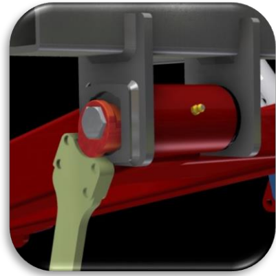
Hold adjuster with spanner whilst tightening Nylon Insert nut
