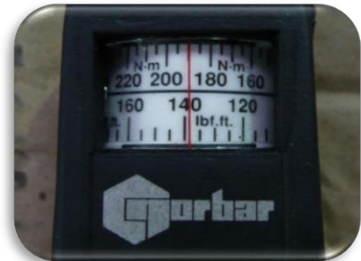
Torque Nylon Insert nut to 190N.m (140lbf.ft)
