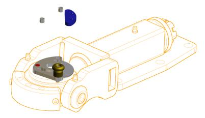
5. Place the cover plate on top of the assembly with all holes lined up – including the dust guard and bolt holes. Also ensure at this point the secondary lock spindle is returning after depressed ensuring spring action.
