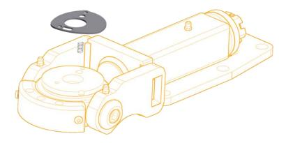
3. Next, position the pre-assembled lock plate over the washer making sure all holes are lined up through to the universal.
