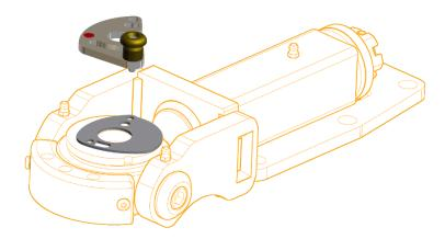
4. Fit the bolt sleeves through the locking plate in line with the threaded holes in the universal. Also place the poly dust guard on the washer plate with the two small locating bosses facing up.
