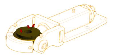
2. Once the holes are clear, the first step is to place the plunger spring in its location hole the universal. Position the washer plate on the universal ensuring all holes are lined up.
