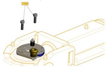
7. Check operation of lock assembly and confirm operation with tow pin.
