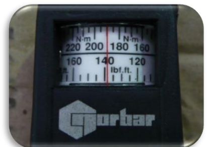
Torque Nylon Insert nut to 190N.m (140lbf.ft)
