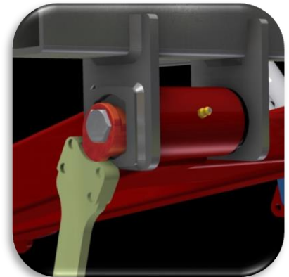
Hold adjuster with spanner whilst tightening Nylon Insert nut
