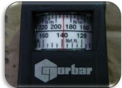
Torque Nylon Insert nut to 190N.m (140lbf.ft)
