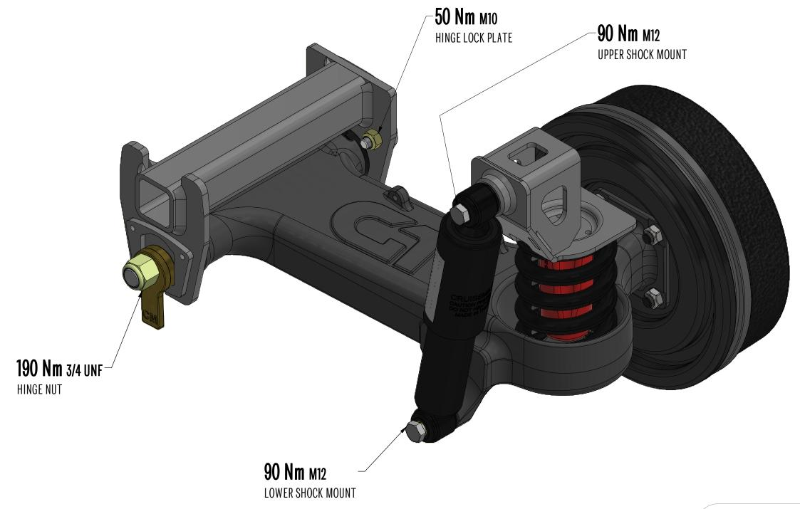
USE SPECIFIED NYLOC INSERT NUTS ONLY (GRADE 5 OR CLASS 8)
