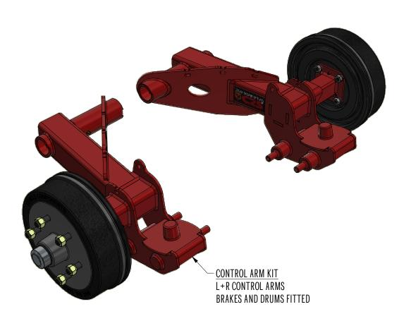
(E) BRAKE . STUD PATTERN OPTION CONDITIONS (E) ELECTRIC Ε HYDRAULIC VT ONLY Н
